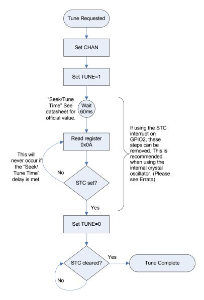
**Figure 14. Channel Selection Flowchart**
