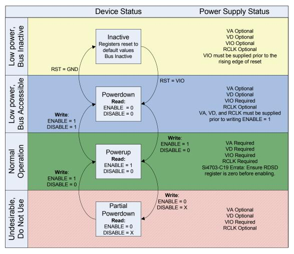
Figure 2. Powerup, Powerdown, and Reset State Diagram
