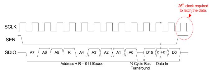
Figure 5. 3-Wire Control Interface Read Timing Diagram
