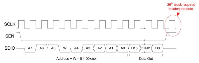
Figure 4. 3-Wire Control Interface Write Timing Diagram
