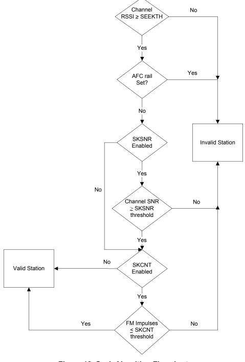
Figure 18. Seek Algorithm Flowchart
