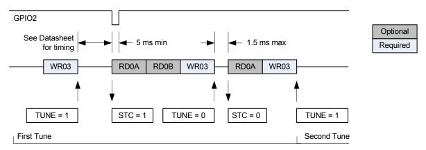
**Figure 13. Channel Selection Timing**
