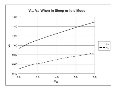
When the device is active (not in sleep or idle mode), the input voltage thresholds are different, depending on the state of TTLenable (bit 3) within the I2C\_Address byte stored in the Configuration zone of the EEPROM. When a common voltage is used for the ATSHA204  $V_{CC}$  pin and the input pull-up resistor, then this bit should be set to a one, which permits the input thresholds to track the supply as follows:
