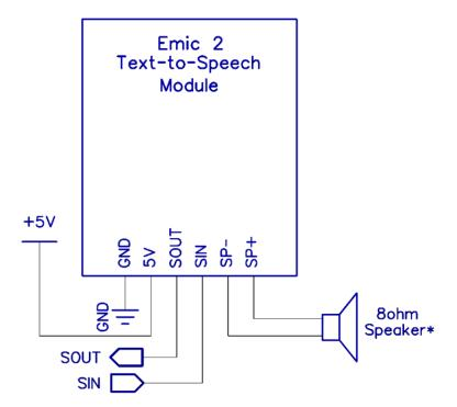
\*Note: For audio output, a connection needs to be made to either SP+/SP- or the 1/8" audio jack. Audio quality may be affected if both outputs are used at the same time.
