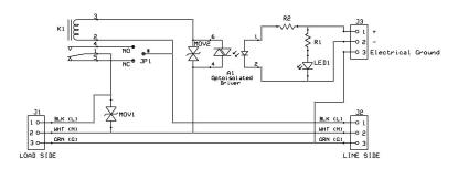
Jumper wire JP1 is between NO and \* for normally open operation or between NC and \* for normally closed operation. Soldering is required to rewire the unit.
