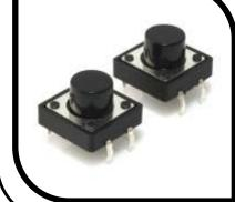
This is included because an Arduino doesn't sense the same way we do (ie button pressed, button unpressed). Instead it looks at the voltage on the pin and decides whether it is HIGH or LOW. The button is set up to pull the Arduino's pin LOW when it is pressed, however, when the button is unpressed the voltage of the pin will float (causing occasional errors). To get the Arduino to reliably read the pin as HIGH when the button is unpressed, we add the pull up resistor.
