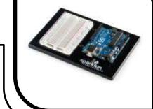
everything in. Once the circuit is assembled you'll need to upload the program. To do this plug the Arduino board into your USB port. Then select the proper port in **Tools > Serial Port > (the comm port of your Arduino)**. Next upload the program by going to **File > Upload to I/O Board (ctrl+U)**. Finally, bask in the glory and possibility that controlling lights offers.
