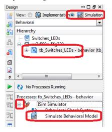
The simulation will be compiled, and then the simulator tool is launched. On start-up the simulator will simulate the first microsecond:
