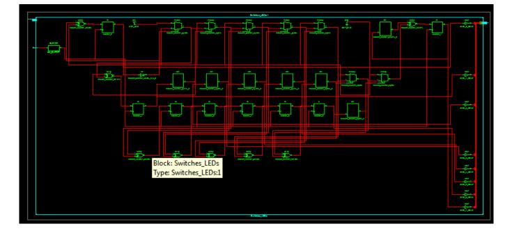
• The Routed Design, which shows the physical locations and interconnects that are used on the FPGA chip:
