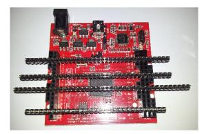
The LogicStart MegaWing has been designed especially for people starting out with FPGAs, converting the Papilio One into something that matches the features and accessibility of the FPGA boards developed for the education market. When mated with a Papilio One, it adds a few nice extras that will appeal to the Papilio One's target market, such as a small joystick, 8 channel ADC, and a 3.5mm audio jack.
