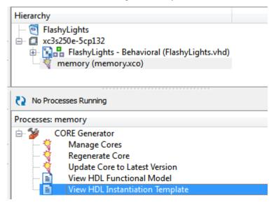
Add it to the source, connecting the top 10 bits of the counter to the ROM's address bus (addra), and the data bus (douta) to the LEDs:
