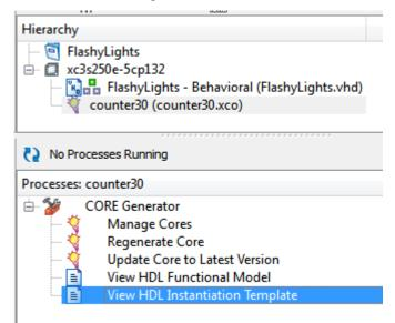
Copy and paste the useful bits into your top level project - add a signal "counter" to be connected to the output of the counter. Here's the completed source:
