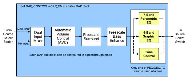
Figure 12. Digital Audio Processing Block Diagram
