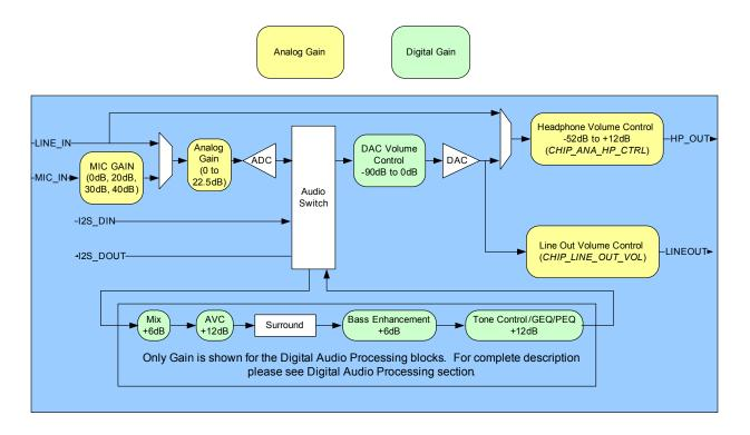
Figure 2. SGTL5000 Simplified Internal Block Diagram
