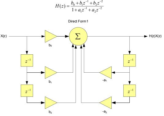
Figure 15. 5-Coefficient Biquad Filter and Transfer Function
