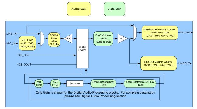
Figure 8. System Block Diagram, Signal Flow and Gain
