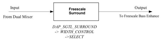
The Freescale Surround can be enabled or configured in pass-through mode (input is passed through without any processing). When enabling the Surround, mono or stereo input type must be selected based on the input signal. Surround width may be adjusted for the size of the sound stage.
