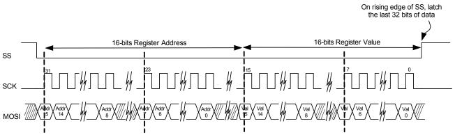
Figure 18. Functional Timing Diagram of SPI Protocol
