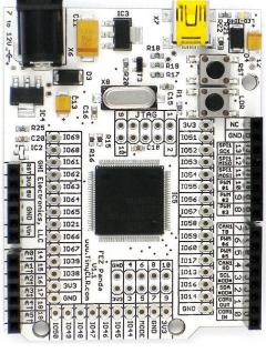
\* These pins can work as interrupt inputs \*Di2 and Di3 are open drain pins with 2.2K pull up resistors.
