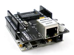
To use multiple shields, we need to make sure they are not using the same pin. This can be accomplished by looking at the schematics of each shield. A simpler option is to create a project and include the driver files of all shields. If the shields are using the same pins then an exception will be raised signaling an error.
