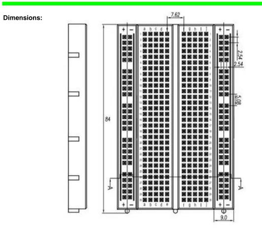
400 tie points clear solderless breadboard(units in mm)
