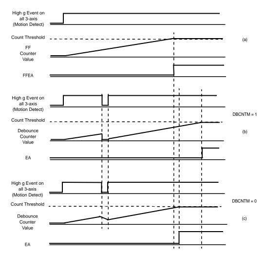
Figure 14. DBCNTM Bit Function
