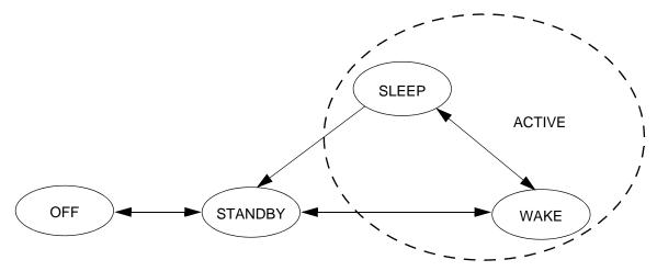
Figure 6. MMA8452Q Mode Transition Diagram
