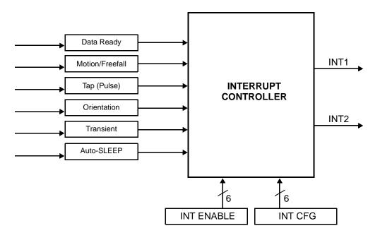
Figure 11. System Interrupt Generation Block Diagram
