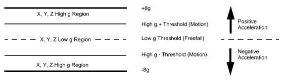
Figure 13. FF\_MT\_CFG High and Low g Level
