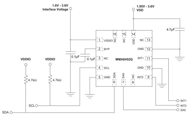
Figure 4. Application Diagram
