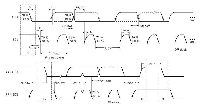
Figure 5. I<sup>2</sup>C Slave Timing Diagram
