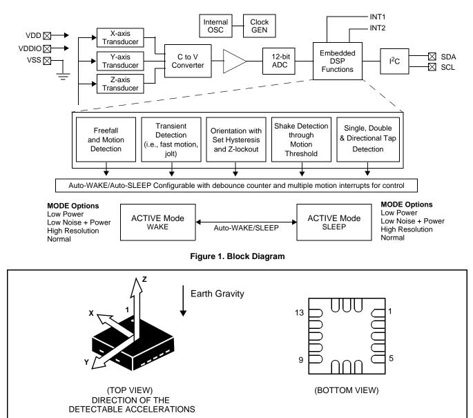
Figure 2. Direction of the Detectable Accelerations
