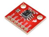
Humidity Sensors make use of a conductive polymer to measure relative humidity. If that polymer gets too dry (or over-saturated) the sensor won't function properly, but that can be reversed.
