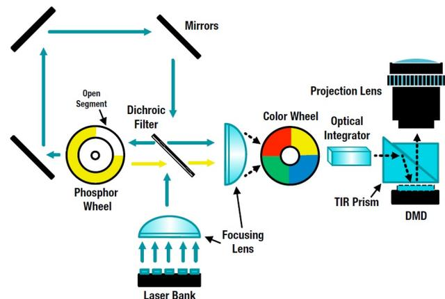
Figure 2-5. Simplified Diagram of a Laser Phosphor Optical Module
