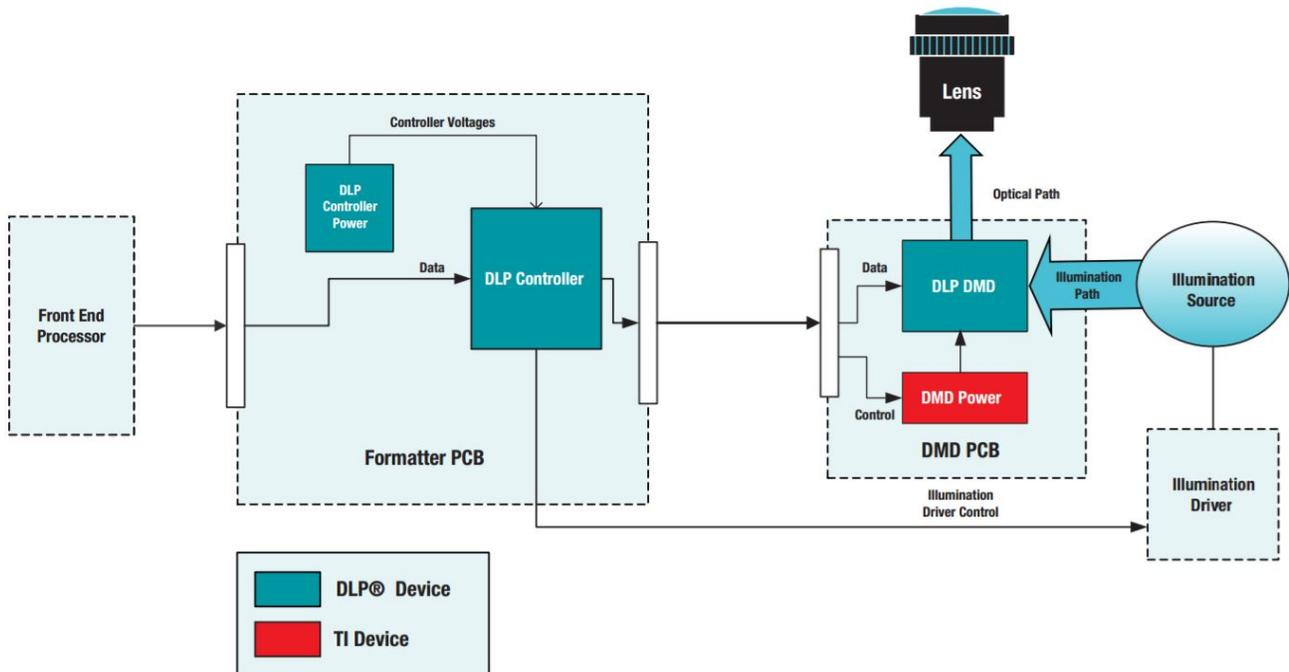
Figure 3-4. Block Diagram of a Typical 4K UHD DLP® Display System
