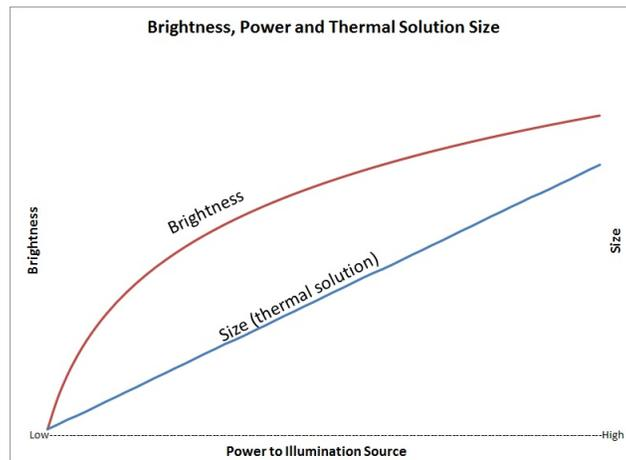
**Figure 4-1. The Tradeoffs Between Brightness, Size, and Power Consumption**
