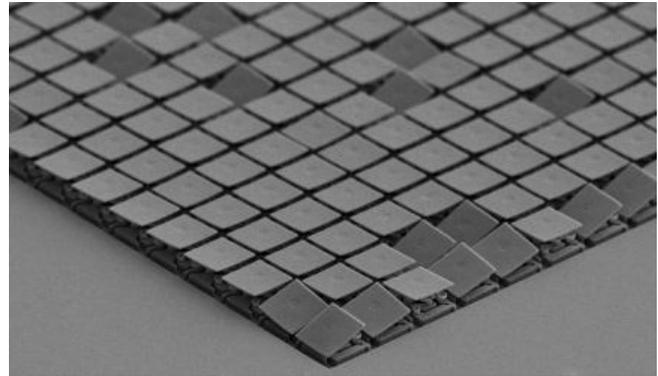
Figure 2-2. Close Up of DMD Micromirrors
