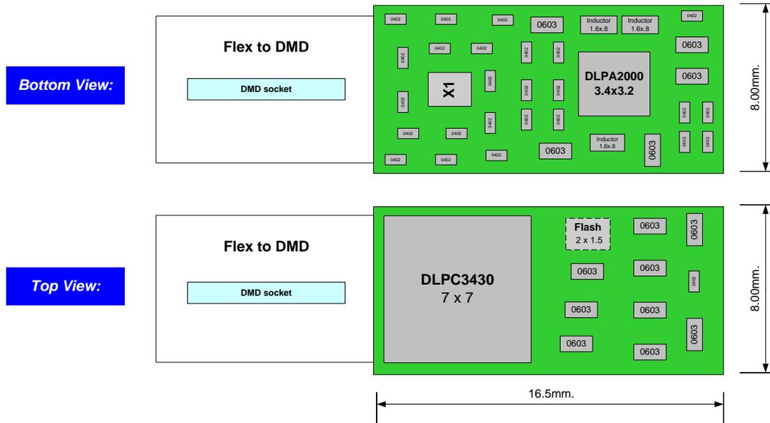
**Figure 3-2. Example of a Small Board Design**
