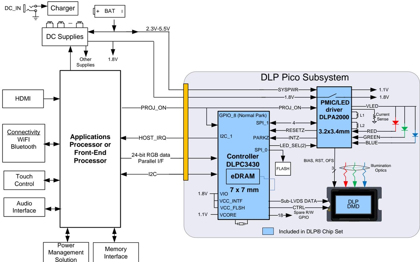
**Figure 3-1. Block Diagram of a Typical DLP® Pico™ System**
