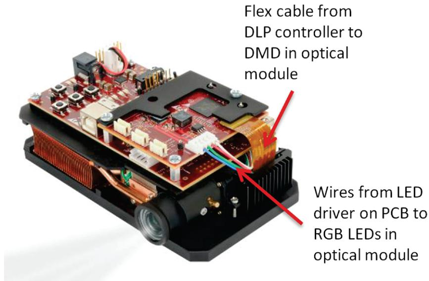
Figure 3-3. DLP® Pico™ Evaluation Module (EVM) With Optical Module and System Electronics
