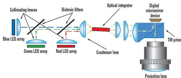
Figure 2-4. Simplified Diagram of an LED Optical Module
