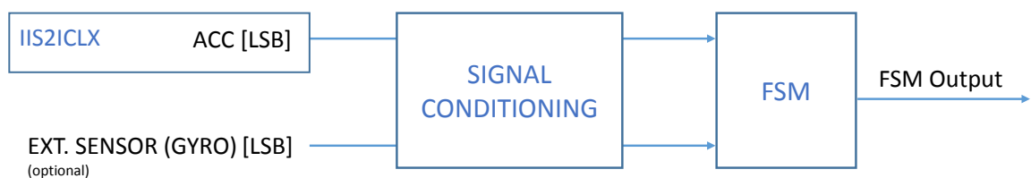
Figure 2. State machine in the IIS2ICLX
