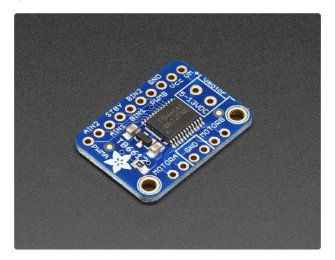
Fire four solenoids, spin two DC motors or step one bi-polar or uni-polar stepper with 1.2A per channel using the TB6612. These are perhaps better known as "the drivers in our assembled Adafruit Motorshield (http://adafru.it/1438) or Motor HAT (https://adafru.it/eRq)" We really like these dual H-bridges, so if you want to control motors without a shield or HAT these are easy to include on any solderless breadboard or perma-proto.
