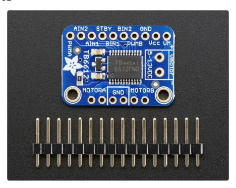
This motor driver is a fairly simple breakout of the TB6612 motor chip, so do check out the datasheet for the TB6612 for any details you need about pin voltage limits, capacitance, etc! (https://adafru.it/emK)
