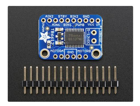
Comes as one assembled and tested breakout plus a small strip of header. You'll need to do some light soldering to attach the header onto the breakout PCB. Arduino, motors, and power supply not included.
