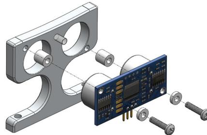
**Step 4:** Mount the PING))) Protector Stand and Sensor to your robot. Two holes in the base of the stand are drilled to accommodate size 6-32 screws (not included).
