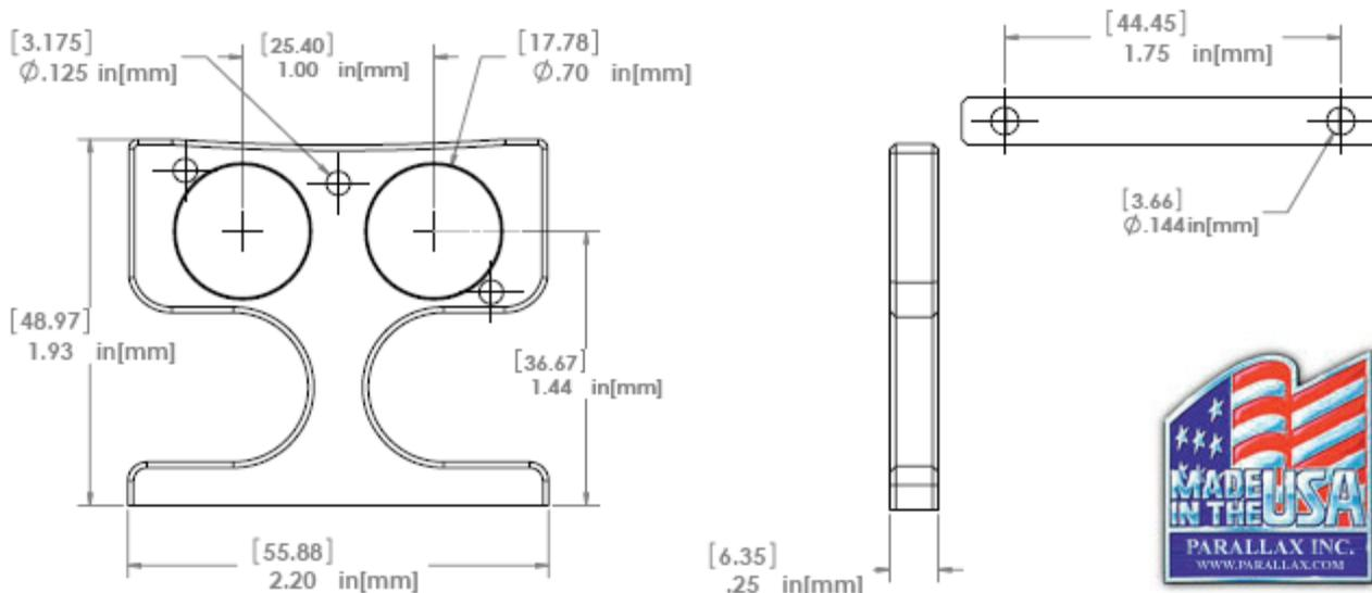
**Step 1:** Place stand on a flat surface with tapped holes facing up. Place a tiny dab of glue on the side (not the flat end) of the light pipe, about a quarter of the way up from the end. Insert light pipe into the hole so that its end is flush with the stand front. The light pipe will project a little less than 1/4" from the back of the stand.
