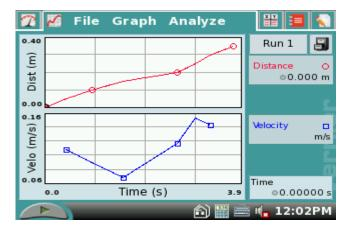
6. The position vs. time graph should be linear and the velocity vs. time graph horizontal. The displacement should correspond to the distance between the first and last black bands.
