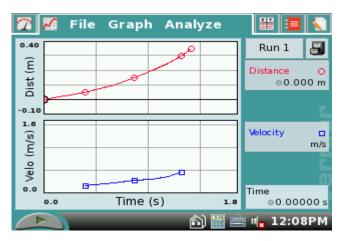
10. Position vs. time and velocity vs. time graphs are shown. As the wheel slows down, the velocity gets smaller and the position does not increase as much. The graphs should be consistent with motion of an object that is undergoing negative acceleration while still moving in a positive direction.
