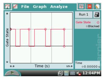
6. The sample graph was created with the index finger entering the beam first. From the graph you can tell that the spacing between the index finger and the middle finger is less than the spacing between the pinky finger and the ring finger. The middle and ring fingers blocked the beam the longest, followed by the index finger, and the pinky finger.
