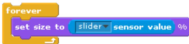
Double-click on the script to run it, and watch. You should see the red & green lights on the PicoBoard start to flash, and as you move the slider, you should notice the size of the Sprite change.
