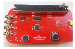
(The red / green lights indicate data is being received (RX) and transmitted (TX) between the PicoBoard and your computer.)
