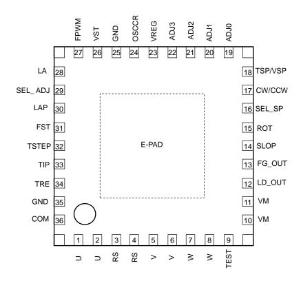
Note 1: Design the pattern in consideration of the heat design because the back side (E-PAD (3.4 mm × 3.4 mm)) and the four corners of the PAD have the role of heat radiation. (The back side (E-PAD) and the four corners of the PAD should be connected to GND because they are connected to the back of the chip electrically.)
