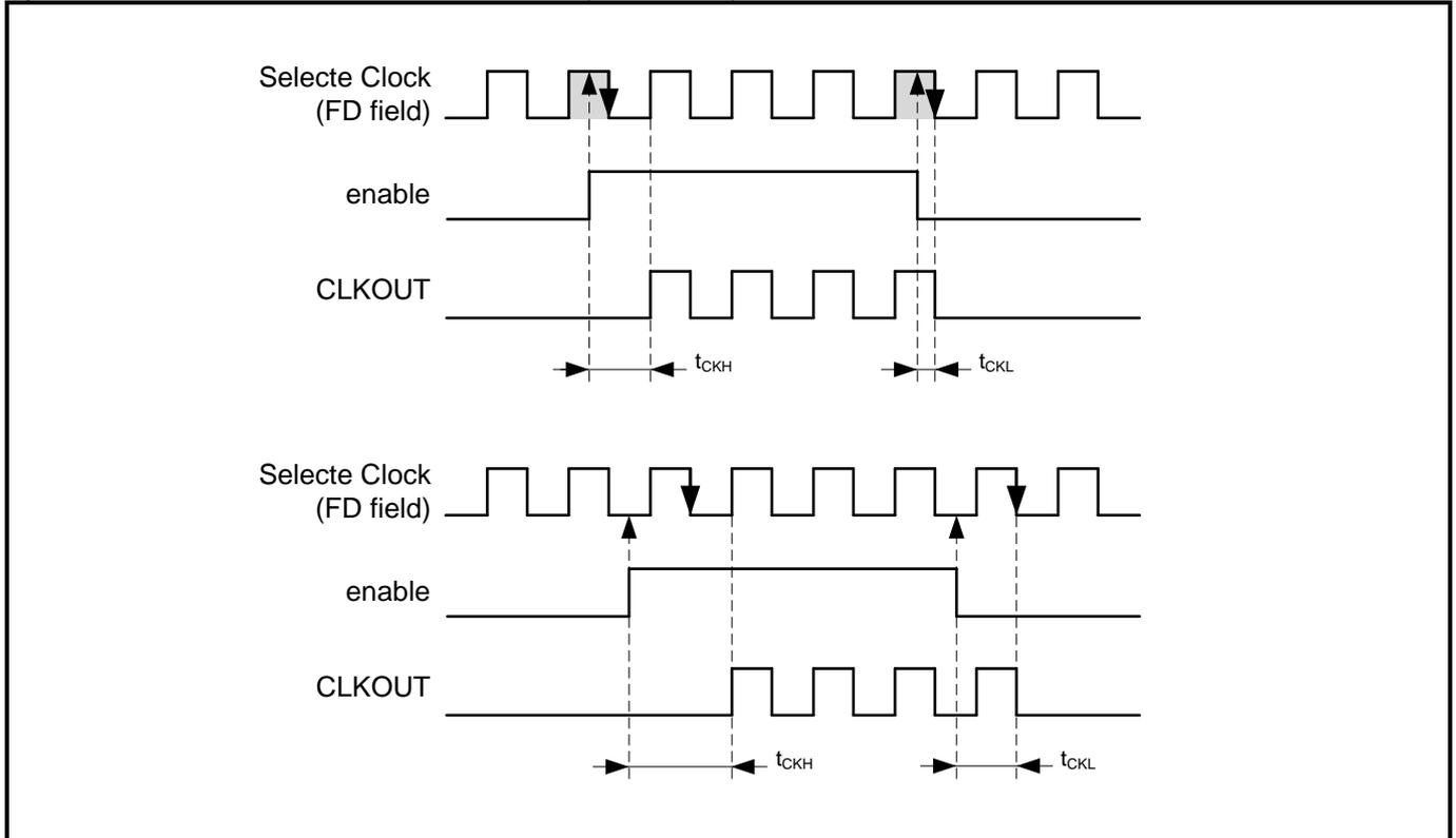
Hint: Glitch free frequency change on CLKOUT requires clearing flag CLKF and bit CLKOE to 0 before the new clock is selected in FD field.
