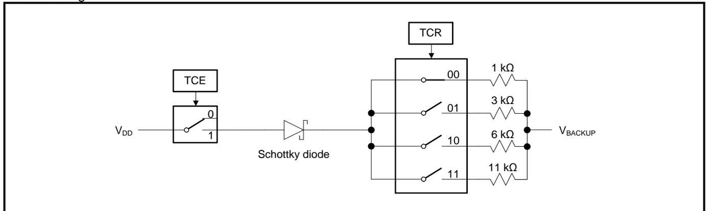
The trickle charger is disabled when the device is in VBACKUP Power state.
