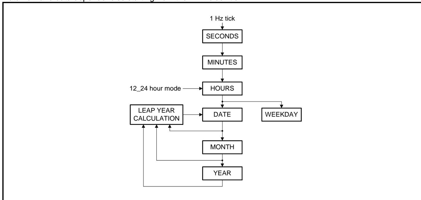
During read/write operations, all clock and calendar registers (00h to 06h) are blocked for 950 ms second. The clock counter increment (1 Hz tick) is inhibited during I<sup>2</sup>C access to the RV-3028-C7 to allow coherent data values. A counter increment (maximum one 1 Hz tick) occurring during inhibition time is memorized and will be realized after the I<sup>2</sup>C stop condition.
