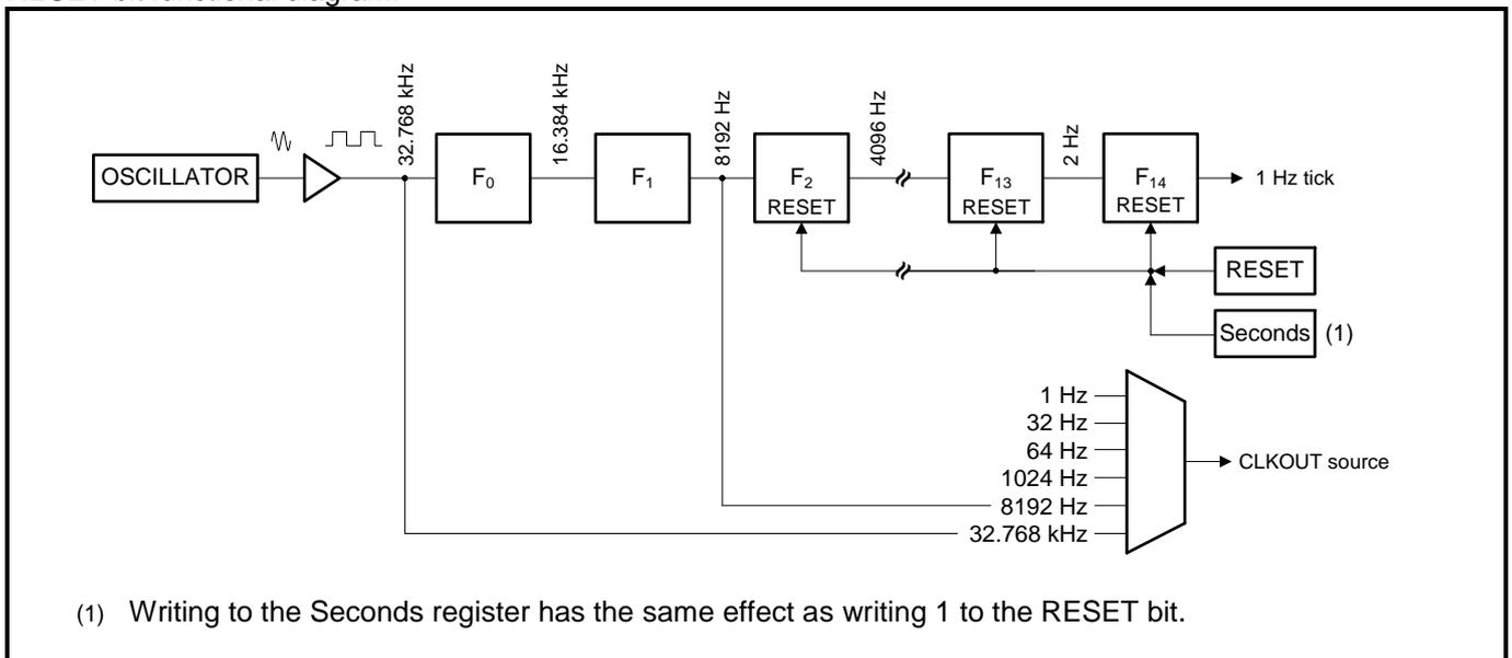
The clock and calendar can be set (in < 950 ms) and then synchronized by writing 1 to the RESET bit.
