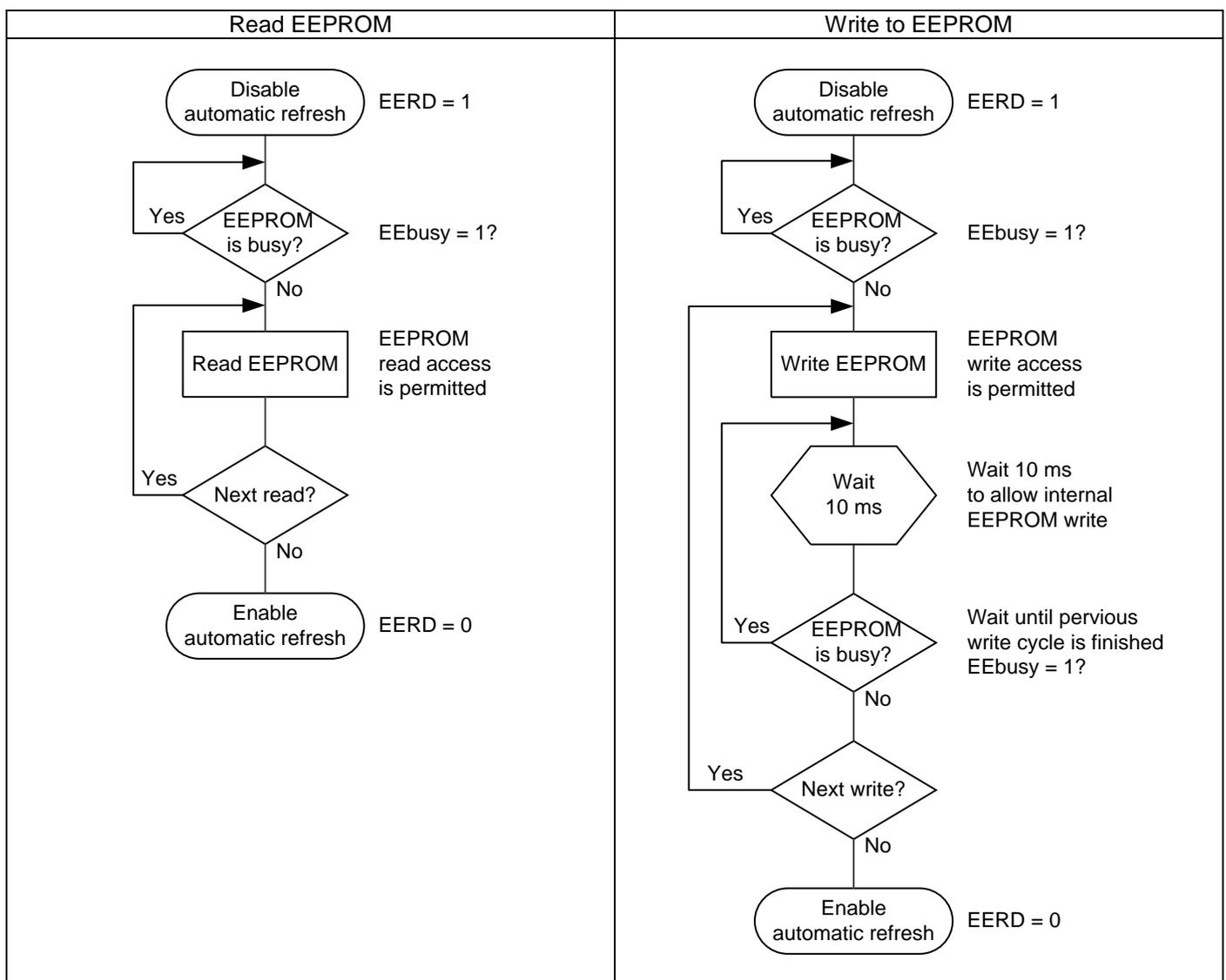
Note: In VDD Power state a minimum voltage of  $V_{PROG} = 1.5\text{ V}$  during the whole EEPROM write procedure is required; i.e. until EEBusy = 0.
