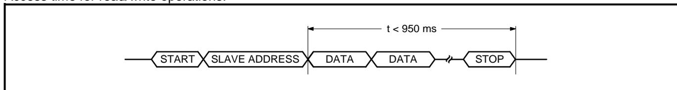
Because of this method, it is very important to make a read or write access in one go, that is, setting or reading seconds through to years should be made in one single access. Failing to comply with this method could result in the time becoming corrupted.
