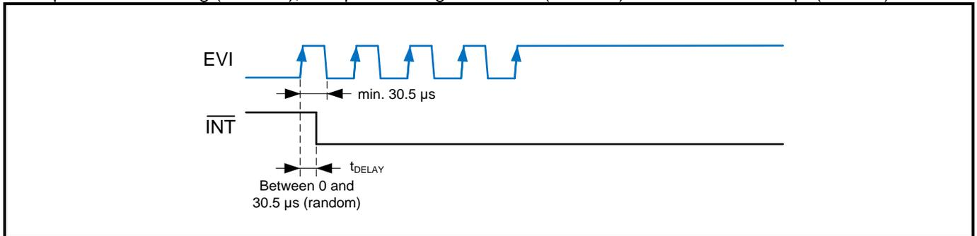
Example with digital debounce filtering ( $ET = 01, 10$  or  $11$ ; sampling period  $t_{SP} = 3.9$  ms,  $15.6$  ms or  $125$  ms), with positive edge/level detection ( $EHL = 1$ ) and enabled interrupt ( $EIE = 1$ ):
