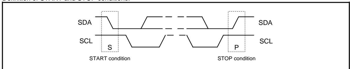
A START condition which occurs after a previous START but before a STOP is called a Repeated START condition, and functions exactly like a normal STOP followed by a normal START.
