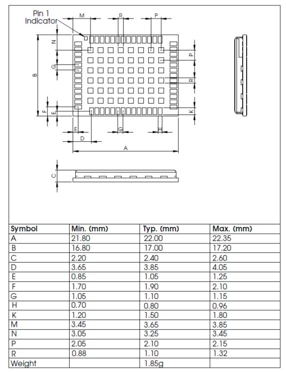
Figure 5: ZED-F9T mechanical drawing
