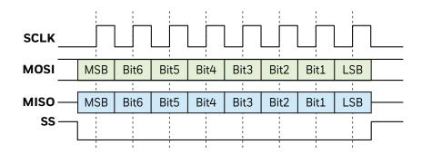
Once the clocking begins, the MPR Series SPI sensor is designed to output up to 4 bytes of data. The first data byte is the Status Byte (8-bit) and the second to fourth bytes are the compensated pressure output (24-bit).
