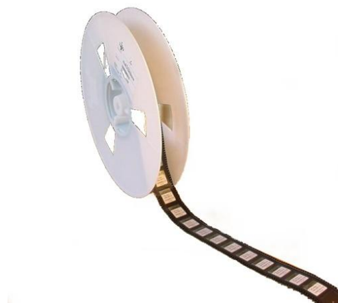
Figure 15: Reeled SARA-U2 modules
