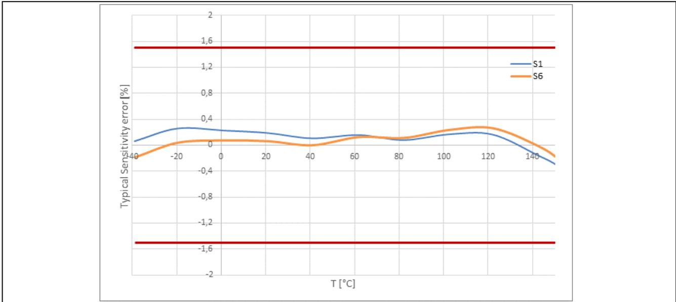
Figure 8 Typical error in sensitivity over temperature
