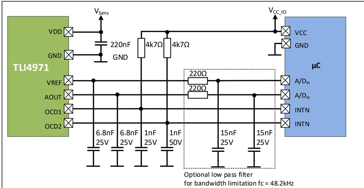
Figure 7 Application circuit with external components
