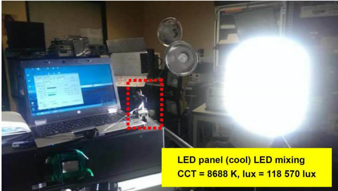
Fig. 8 - VEML6075 Test Set-Up Using a White LED as Light Source
