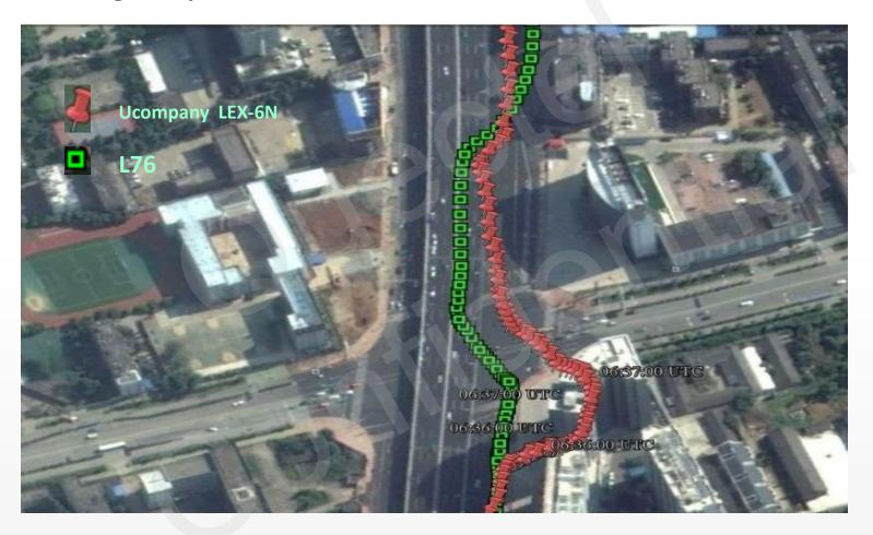
When driving across overpass and making a turn, L76 module can still capture the accurate tracking data. But Ucompany module has a small drift.
