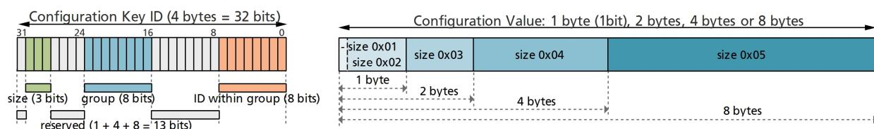
A Configuration Key ID is a 32 bit integer value, which is split into three parts (Note that bits 31, 27..24 and 15..8 are reserved for future use and are currently unused.):
