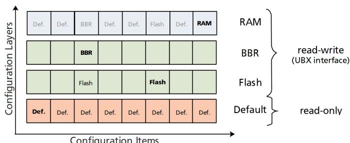
In the example figure above several items (e.g. the first item) are only set in the Default Layer and hence the default value ends up in Current Configuration in the RAM Layer. The third item is present in the Default, Flash and BBR Layers. The value from the BBR Layer has the highest priority and therefore it ends up in the RAM Layer. On the other hand, the default value of the
