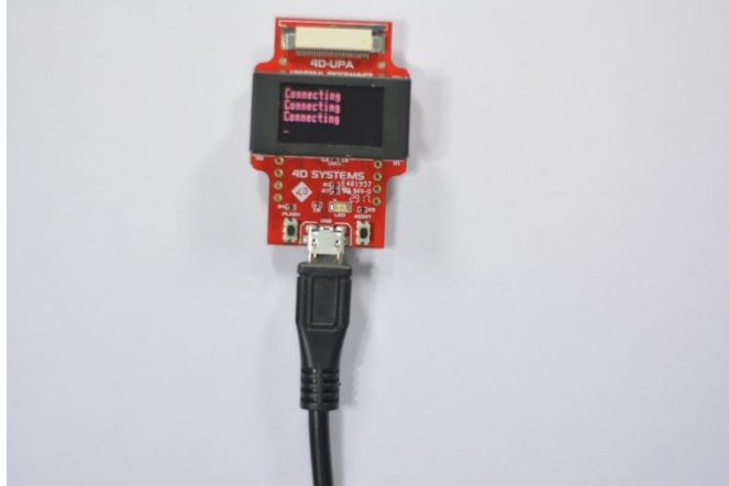
Figure 1. Connection of an IoD-09TH Display module to 4D-UPA with a uUSB Cable.
