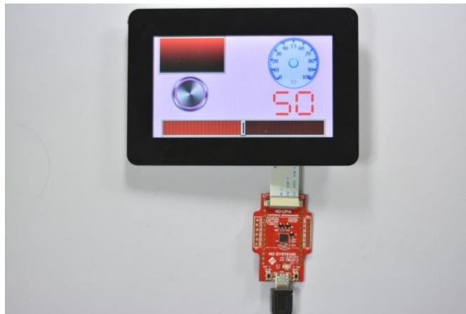
Figure 2. Typical connection of gen4 display module (gen4-uLCD-43DCT-CLB) to 4D-UPA
