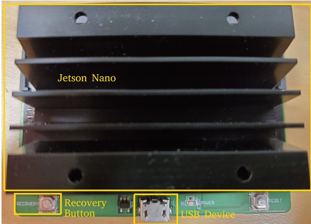
Figure 5: Jetson Nano Flasher board with the Jetson Nano installed
