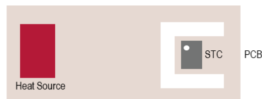
Figure 4: Decoupling the sensor from heat sources
