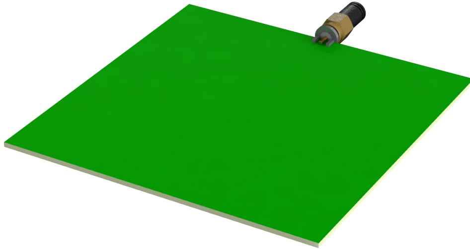
Figure 3. ANT-868-NUB-ccc on Edge of Ground Plane
