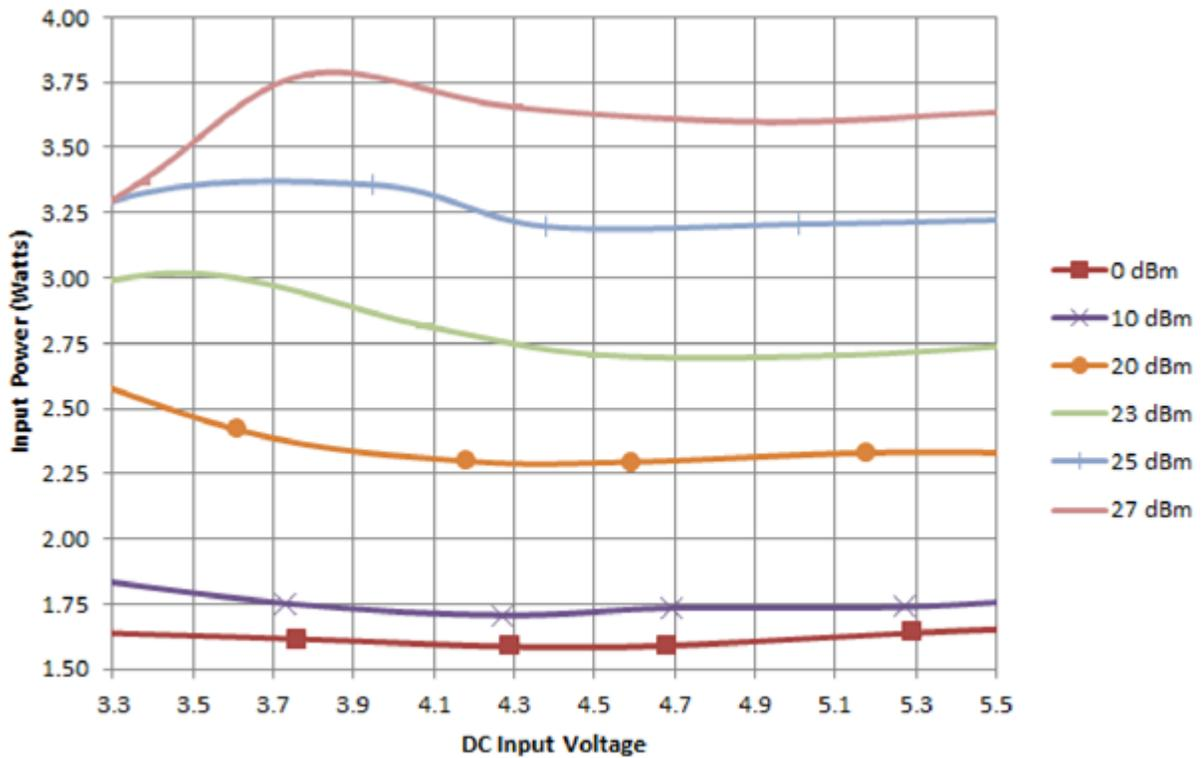
**NOTE:** Power consumption is defined for operation into a 17 dB return loss load (VSWR of 1.33) or better. Power consumption may increase, up to 4 W, during operation into return losses worse than 17 dB and high ambient temperatures. Power consumption will also vary based on which of the [Supported Regions](#) is in use.
