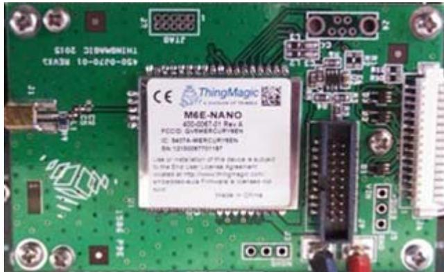
The Nano Carrier Board is an example of a host board to create an assembly that is compatible with the standard Development Kit main board. It has the size and dimensions of the M6e module (69 mm x 43 mm) and uses the same connector for power and control (Molex 532611571 - 1.25mm pin centers, 1 amp per pin rating, which mates with Molex housing p/n 51021-1500 with crimps p/n 63811-0300).
