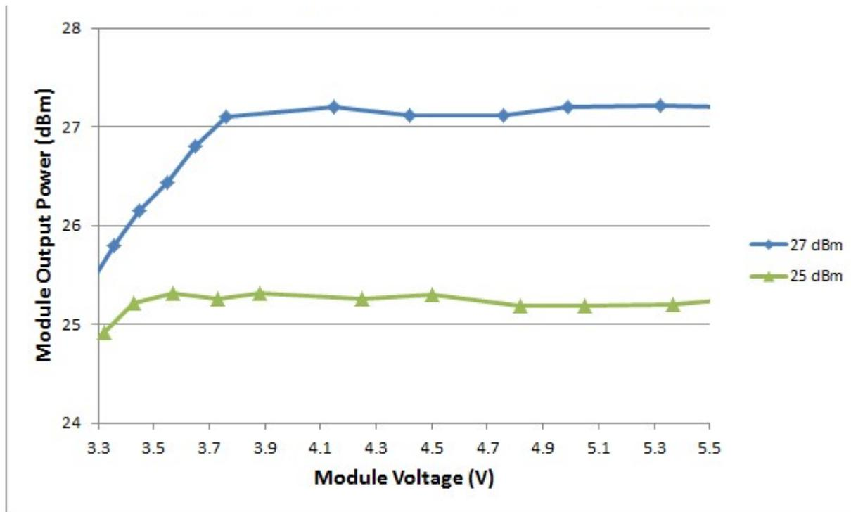
The power drawn by the module is constant, rising slightly as the DC Input Voltage is lowered. Once the 1A input current limit is reached, the input power appears to decrease, but this is because the RF output level is no longer reflecting the desired setting. This chart shows these dependencies:
