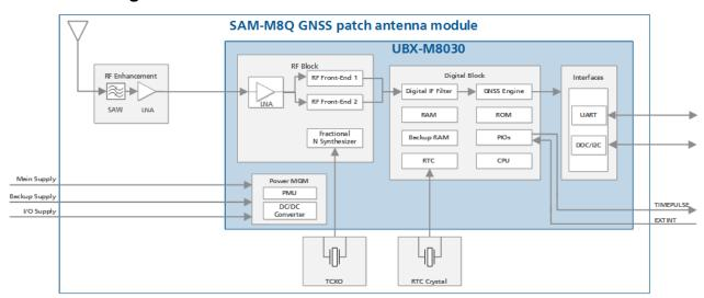
Figure 1: SAM-M8Q block diagram
