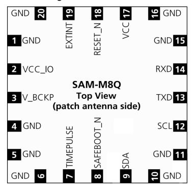
Figure 2: Pin Assignment
