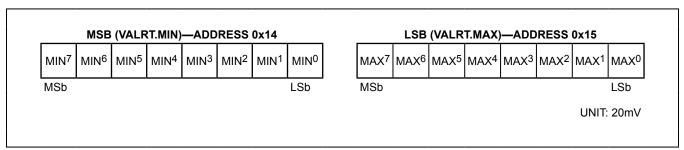
Figure 11. VALRT Register Format
