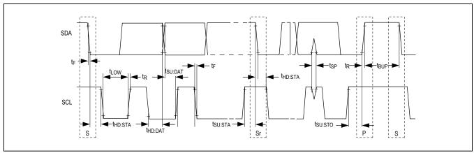
Figure 1. I<sup>2</sup>C Bus Timing Diagram
