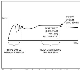
Figure 7. Insertion Waveform Requiring Quick-Start Command
