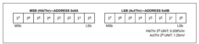
Figure 9. HIBRT Register Format
