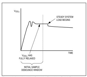
Figure 6. Insertion Waveform Not Requiring Quick-Start Command
