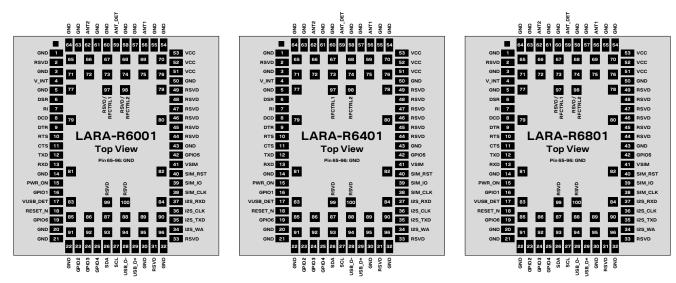
Figure 2: LARA-R6 series pin assignment (top view)
