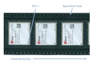
Figure 7: Orientation for LARA modules on tape
