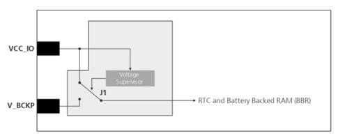
Figure 1: Backup battery and voltage
