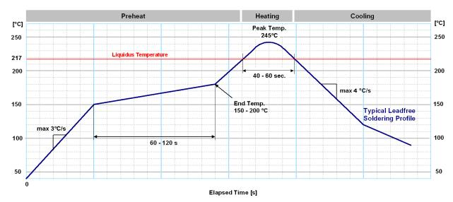
Figure 9: Recommended soldering profile
