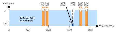
Figure 12: Out-band interference signals
