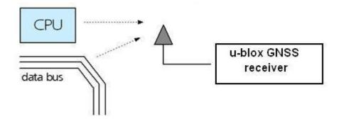
Figure 11: In-band interference sources
