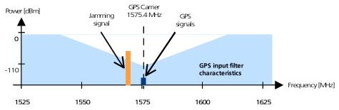
Figure 10: In-band interference signals
