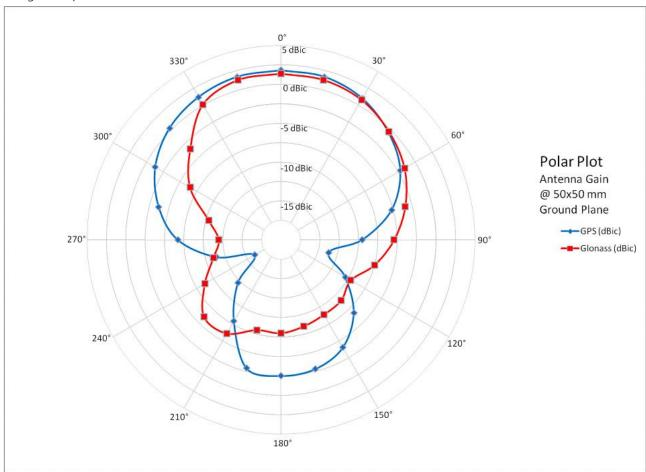
Figure 7: 1.575 GHz typical free space radiation patterns
