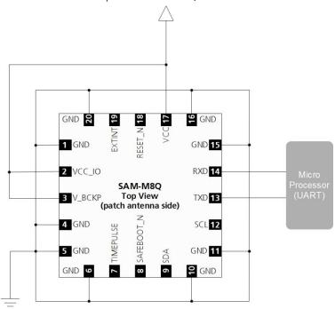
Figure 3: SAM-M8Q GNSS patch antenna design
