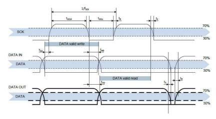
DATA directions are seen from the HTU21D(F) sensor. DATA line in bold is controlled by the sensor. DATA valid read time is triggered by falling edge of anterior toggle.
