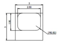
Dimensions are given in mm, tolerances are  $\pm 0.1$ mm. The die pad (thermal center pad) is internally connected to GND.
