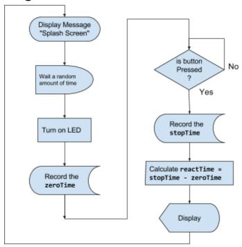
Here is a simple flow chart illustrating the programming for the reaction timer.
