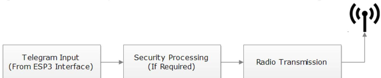
**Figure 6 – Telegram Transmission Flow**
