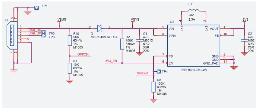
VBUS is the 5V input from the micro-USB port, which is fed through a Schottky diode to generate VSYS. The VBUS to VSYS diode (D1) adds flexibility by allowing power ORing of different supplies into VSYS.
