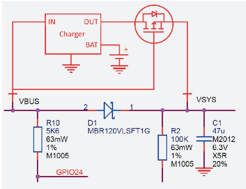
In the example we feed VBUS to the input of the charger, and we feed VSYS with the output via the previously mentioned P-FET arrangement. Depending on your use case you may also want to add a Schottky diode across the P-FET as described in the previous section.
