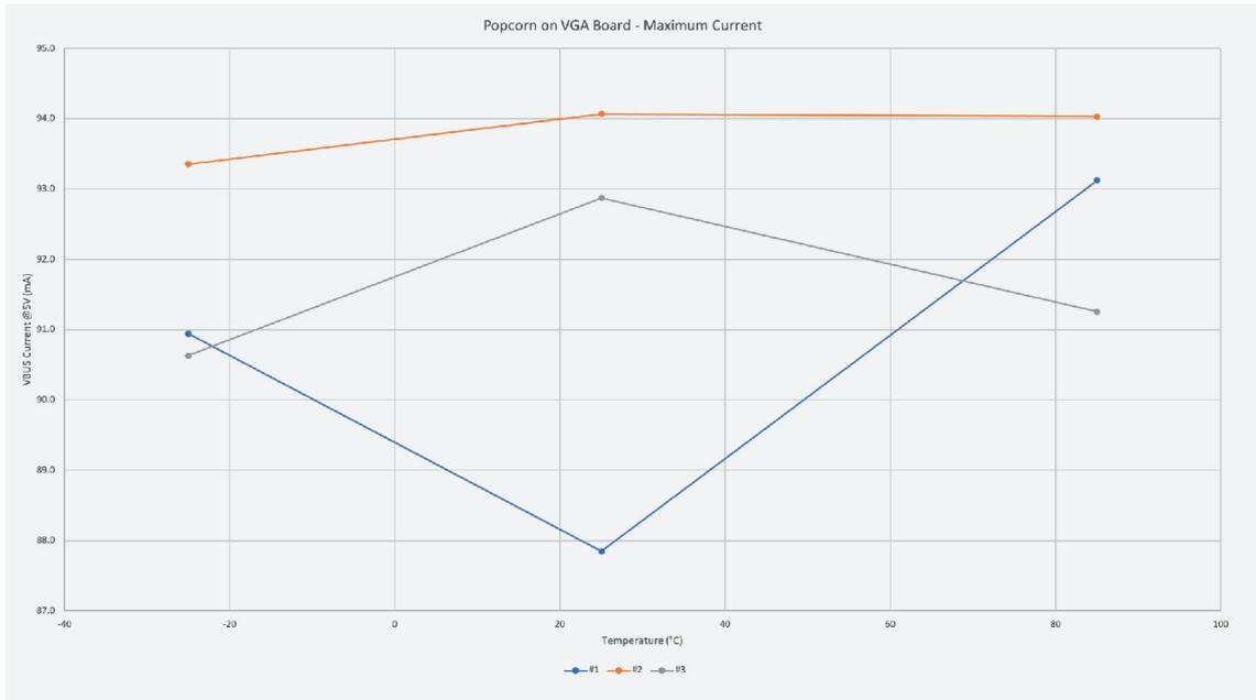
Table 2. Popcorn running on the VGA Board (VGA video, SD Card and I2S audio) with power saving disabled (GPIO23 pulled high)
