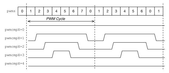
**Figure 12:** Center-aligned PWM waveforms generated from one comparator. All possible waveforms are shown for a 3-bit PWM precision. The signals can be inverted at the GPIOs to generate opposite-phase waveforms.
