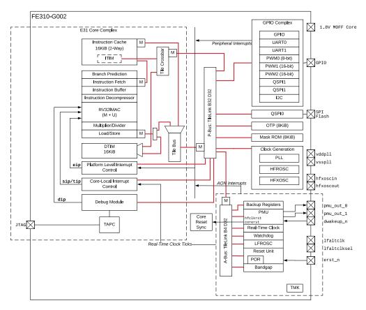
Figure 1: FE310-G002 top-level block diagram.
