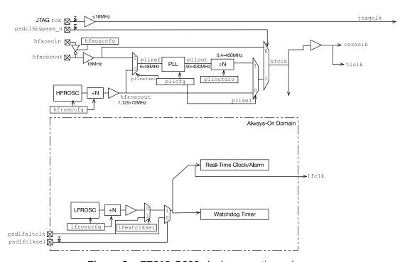
Figure 2: FE310-G002 clock generation scheme
