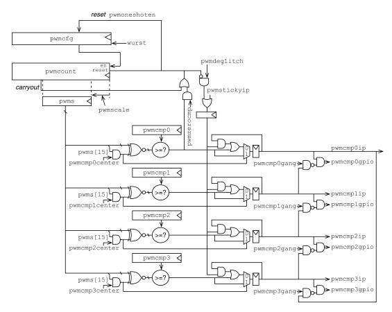
Figure 10: PWM Peripheral
