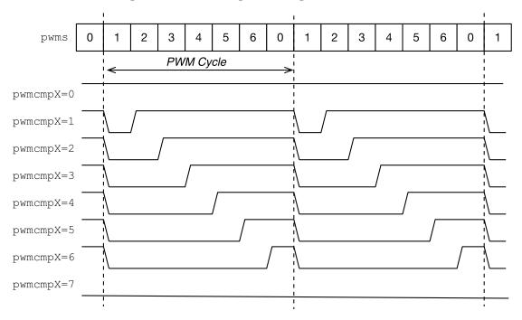
Figure 11: Basic right-aligned PWM waveforms. All possible base waveforms are shown for a 7-clock PWM cycle (pwmcmp0=6). The waveforms show the single-cycle delay caused by registering the comparator outputs in the pwmcmp $\boldsymbol{X}$ ip bits. The signals can be inverted at the GPIOs to generate left-aligned waveforms.
