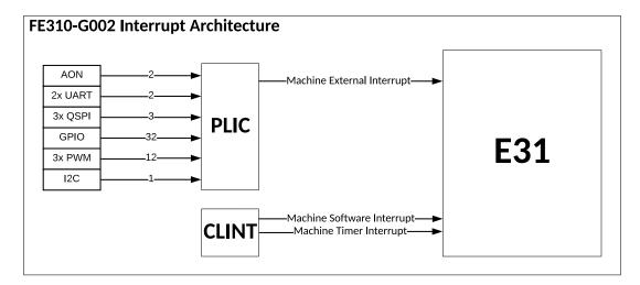
Figure 4: FE310-G002 Interrupt Architecture Block Diagram.
