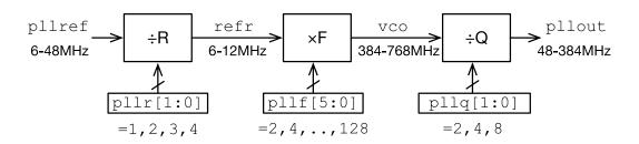
**Figure 3:** Controlling the FE310-G002 PLL output frequency.
