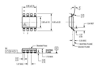
For Reference Only; not for tooling use (reference MS-012AA) Dimensions in millimeters
