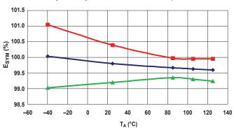
**Total Output Error versus Ambient Temperature**
