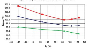
**Total Output Error versus Ambient Temperature**
