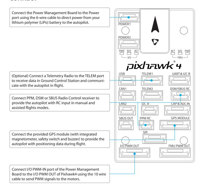
Connect the PMB to the POWER port using the 6-wire cable to direct power from your lithium polymer (LiPo) battery to the autopilot.
