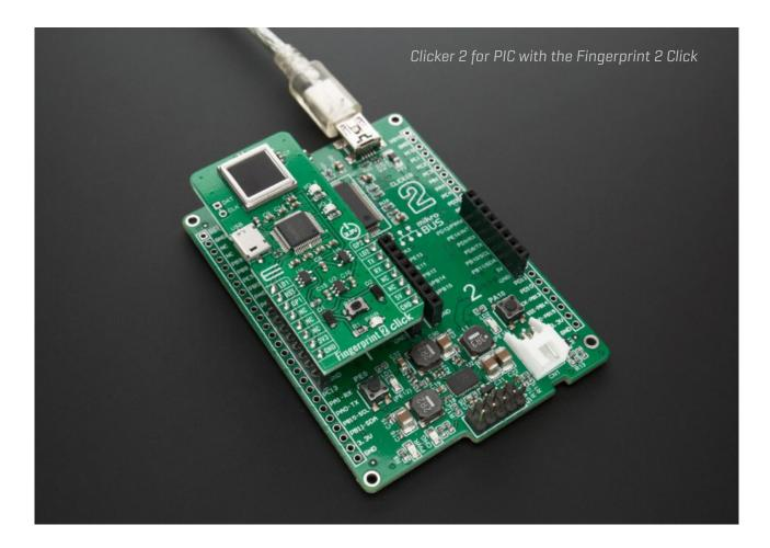
The default communication channel is UART, with also USB (CDC class) supported. The UART baud rate of Fingerprint 2 Click is set to default configuration parameters:
