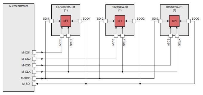
Figure 7-25. Three DRV8889A-Q1 Devices Connected in Parallel Configuration
