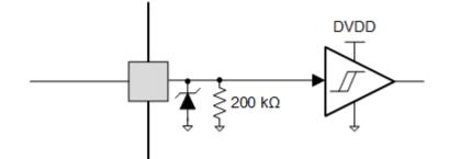
Figure 7-16. Logic-Level Input Pin Diagram
