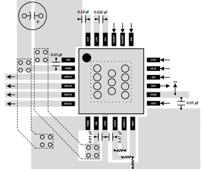
Figure 10-2. QFN Layout Recommendation
