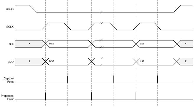
Figure 7-32. SPI Transaction
