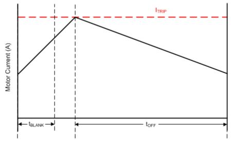
Figure 7-5. Current Chopping Waveform
