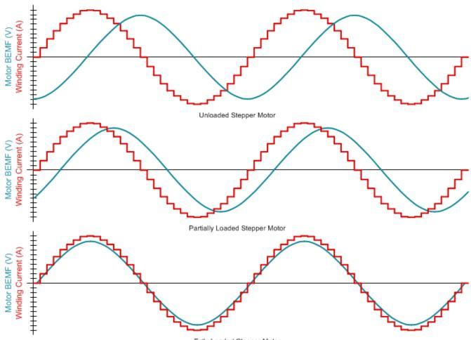
Fully Loaded Stepper Motor
