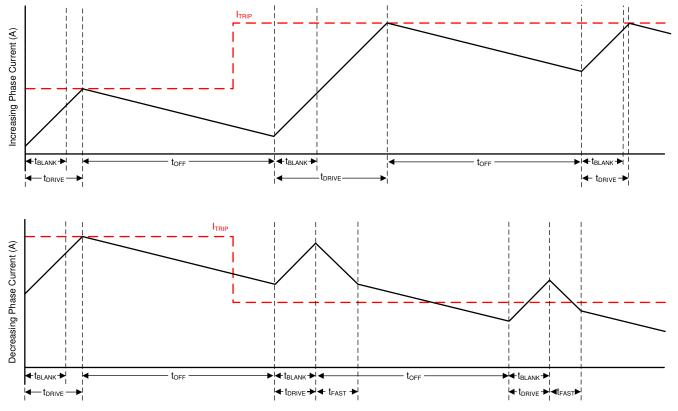
Figure 7-12. Smart tune Dynamic Decay Mode
