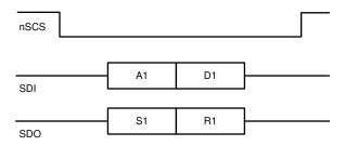
Figure 7-23. SPI Transaction Between MCU and the device
