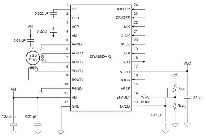
Figure 8-2. Typical Application Schematic (HTSSOP package)
