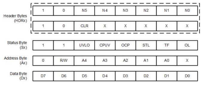
Figure 7-31. Contents of Header, Status, Address, and Data Bytes
