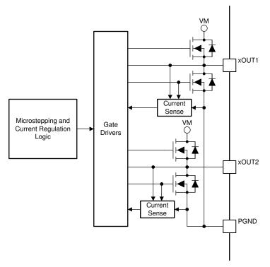
Figure 7-2. PWM Motor Driver Block Diagram
