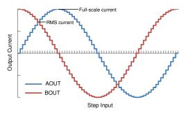
Figure 7-1. Full-Scale and RMS Current
