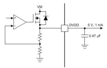
Figure 7-15. Linear Voltage Regulator Block Diagram
