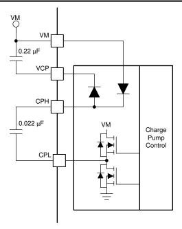
Figure 7-14. Charge Pump Block Diagram
