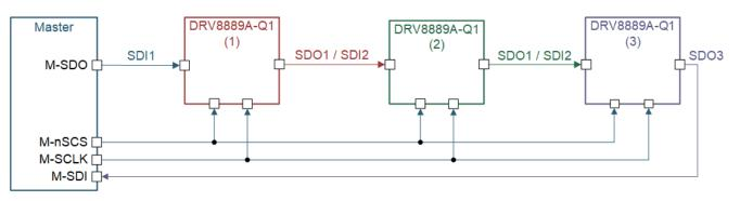
Figure 7-27. Three DRV8889A-Q1 Devices Connected in Daisy Chain
