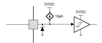
Figure 7-17. Logic-Level with Internal Pull-up Input Pin Diagram
