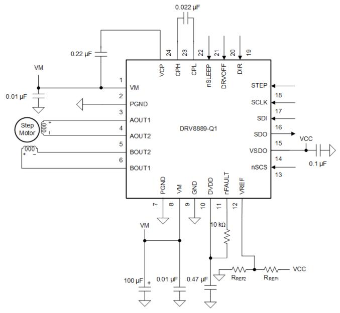
Figure 8-3. Typical Application Schematic (VQFN package)
