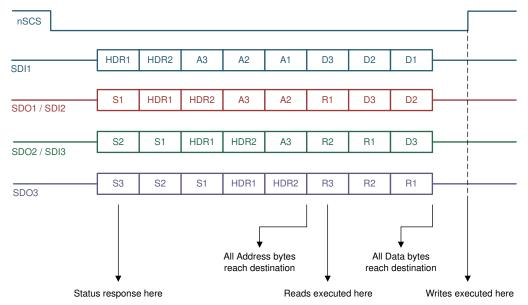
Figure 7-28. SPI Frame With Three Devices
