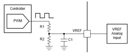
Figure 7-4. Controlling VREF With a PWM Resource
