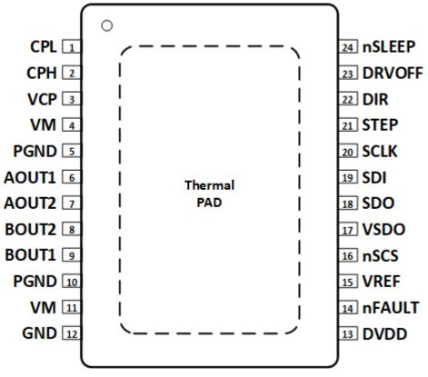
Figure 5-1. PWP PowerPAD™ Package 24-Pin HTSSOP Top View
