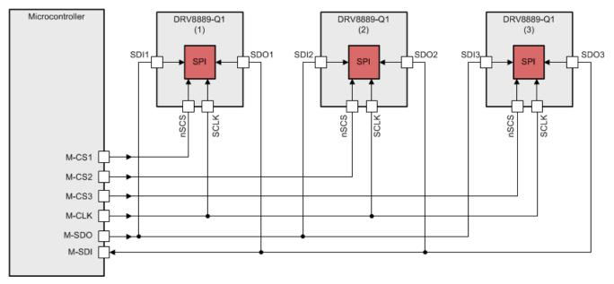
Figure 7-24. Three DRV8889-Q1 Devices Connected in Parallel Configuration
