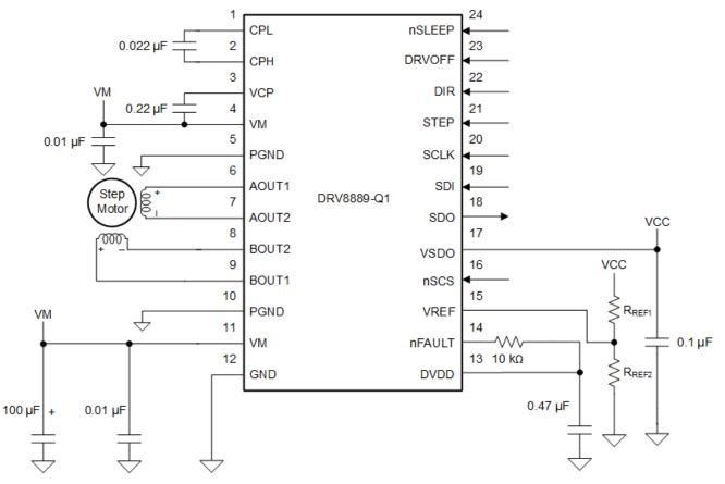
Figure 8-1. Typical Application Schematic (HTSSOP package)
