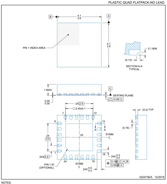
1. All linear dimensions are in millimeters. Any dimensions in parenthesis are for reference only. Dimensioning and tolerancing per ASME Y14.5M. This drawing is subject to change without notice. The package thermal pad must be soldered to the printed circuit board for optimal thermal and mechanical performance.
