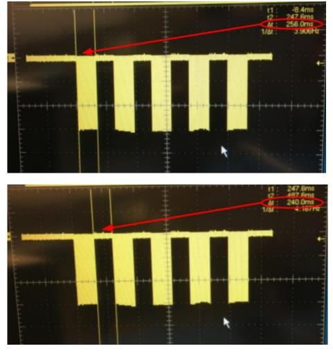
The module needs 2ms RF settling time after ramp up. So, if RF ON time is specified as 2ms or less, RF will not be turned on. 3ms is the least time where RF ON pulse can be seen. For RF ON time>2ms, a compensation of 2ms for settling time is included in FW for accurate timing.
