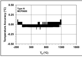
**FIGURE 2-3:** Typical Temperature Accuracy from NIST ITS-90 Database, Type N.
