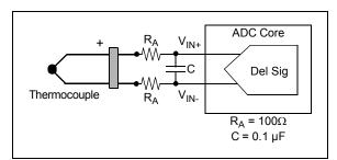
FIGURE 6-7: Adding a Low-Pass Filter.
