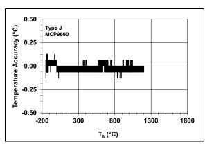
**FIGURE 2-2:** Typical Temperature Accuracy from NIST ITS-90 Database, Type J.
