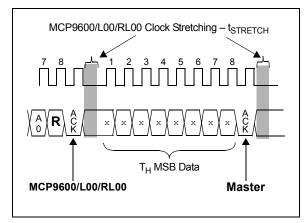
FIGURE 4-2: Clock Stretching.
