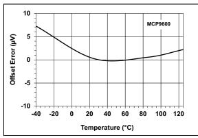
**FIGURE 2-15:** Input Offset Error Voltage  $(V_{IN+}, V_{IN-})$ .
