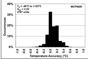
FIGURE 2-23: Cold-Junction Sensor Temperature Accuracy Distribution.
