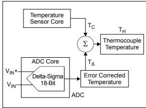
**FIGURE 5-2:** Thermocouple Temperature Register Block Diagram.
