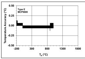
**FIGURE 2-9:** Typical Temperature Accuracy from NIST ITS-90 Database, Type E.
