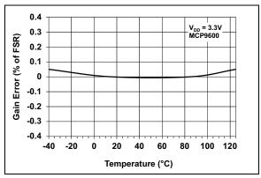
FIGURE 2-18: Full-Scale Gain Error.
