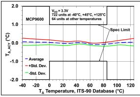
FIGURE 2-20: Cold-Junction Sensor Temperature Accuracy.
