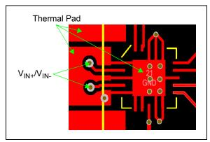
FIGURE 6-1: Recommended PCB Layout.
