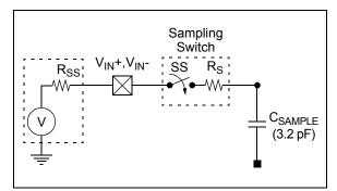
FIGURE 6-5: Thermocouple Input Stage.
