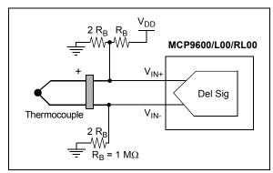
**FIGURE 6-6:** Adding Open-Circuit Detection Resistors.
