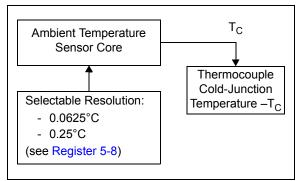
**FIGURE 5-4:** Thermocouple Cold-Junction Register ( $T_C$ ) Block Diagram.
