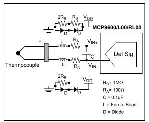
FIGURE 6-9: Adding Ferrite Beads.
