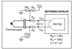
FIGURE 6-8: Adding Open-Circuit
