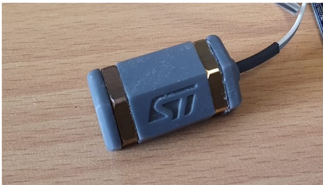
Figure 10. Example of an electrode for water-leak detection
