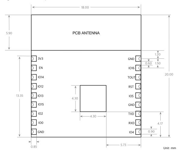
Figure 2-1. Top view of The ESP-WROOM-02
