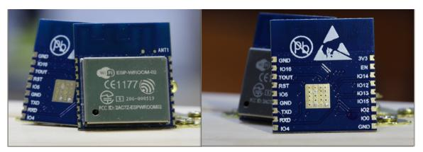
Figure 1-1. ESP-WROOM-02 Module
