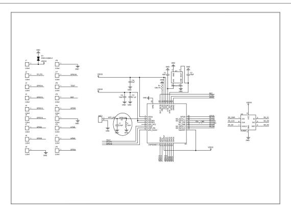
Figure 5-1. ESP-WROOM-02 Schematics
