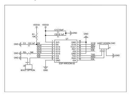
Figure 5-2. ESP-WROOM-02 Peripheral Schematics
