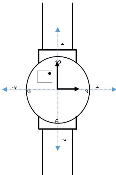
Figure 3: Device co-ordinate system assumed for gesture detection
