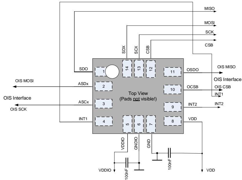
**Primary: 4-wire SPI   Secondary: 3-wire SPI for OIS interface**
