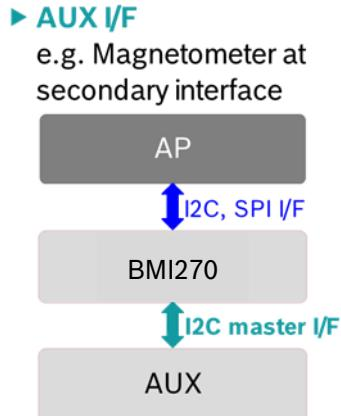
Figure 7: 9-DOF Solution w/ magnetometer (AUX) connected to the 2<sup>nd</sup> I/F
