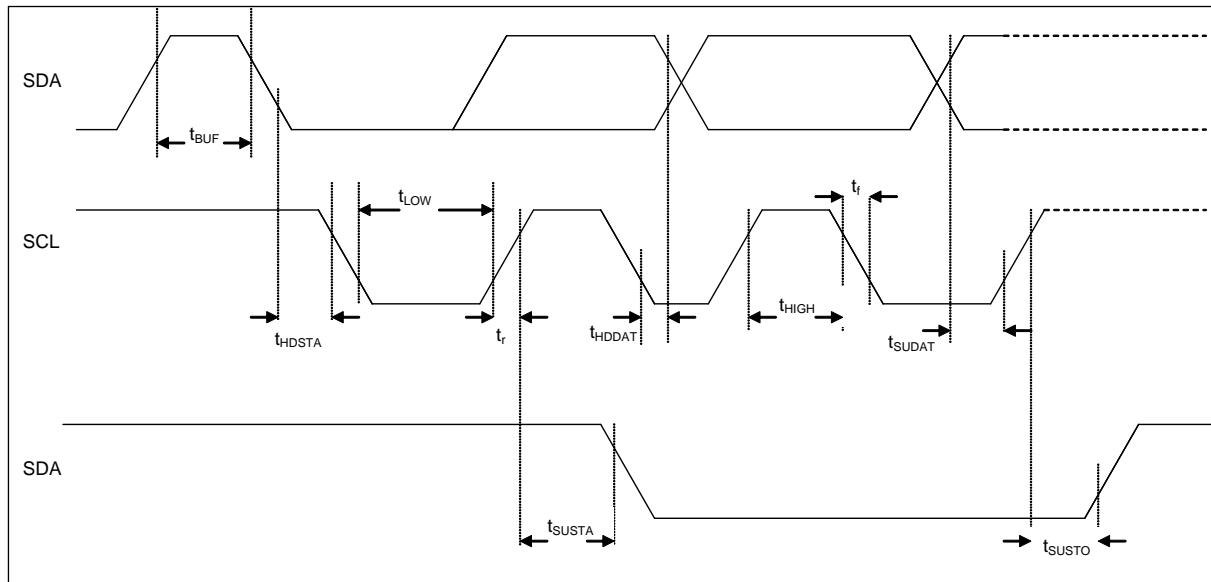
Figure 11: I<sup>2</sup>C timing diagram
