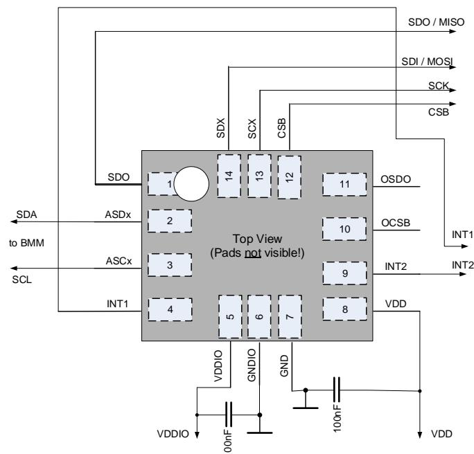
**Primary: I2C Secondary: Auxiliary interface I2C (e.g. BMM150 sensor)**
