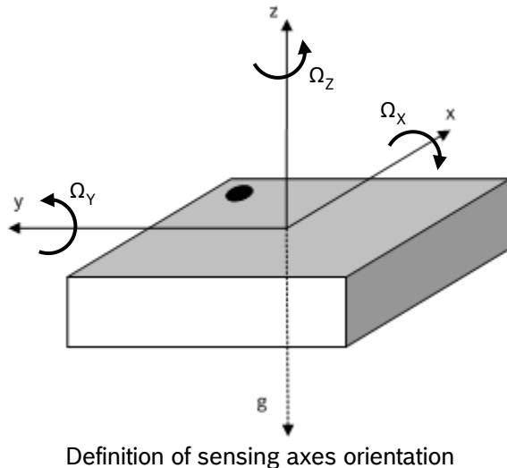
The following table lists all corresponding output signals on X, Y, and Z while the sensor is at rest or at uniform motion in a gravity field under assumption of a  $\pm 4g$  range setting, a 16 bit resolution, and a top down gravity vector as shown above.
