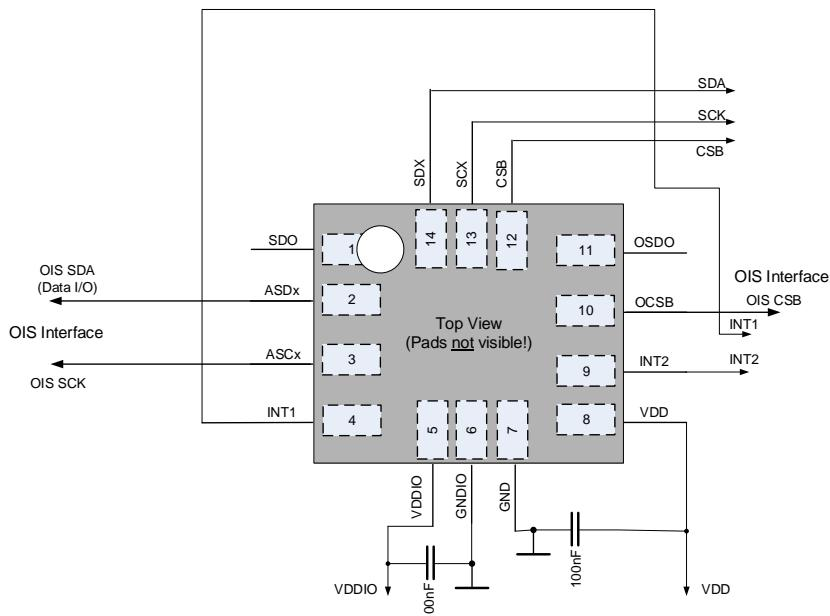
**Primary: 4-wire SPI   Secondary: 4-wire SPI for OIS interface**
